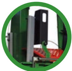
Side feed mounted on bearings, with vertical rest position for transport
