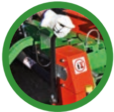
Emergency braking device for models with PTO
