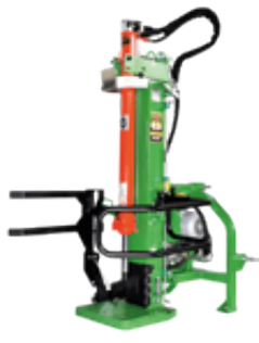
V.PF Fixed PTO pump external tank
