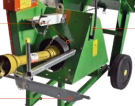
Emergency braking device for models with PTO
