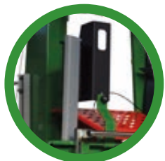
Side feed mounted on bearings, with vertical rest position for transport
