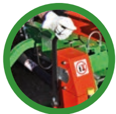
Emergency braking device for models with PTO
